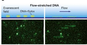
Visualisation of fluorescence-labelled DNA molecules by stretching them with a flow in a combined Magnetic Tweezers TIRF setup.
